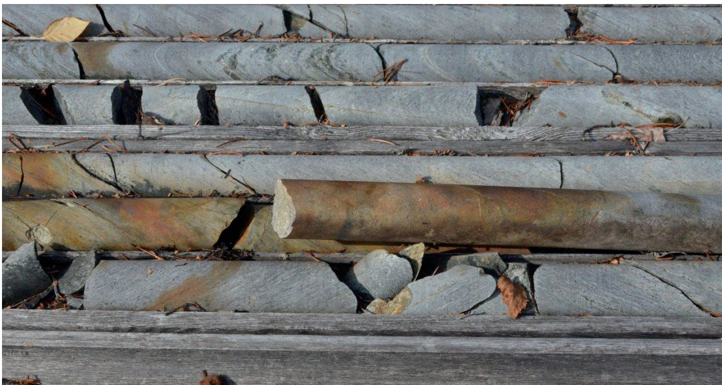
Drill core from 2008 exploration exhibits oxidation of sulphides in unassayed intervals from Relf Zone
